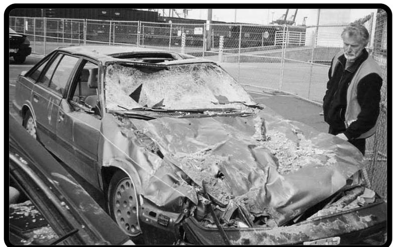
Barry Earl inspects damage to a vehicle parked outside a building with an unreinforced masonry parapet.
