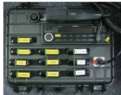
Below: The Stinger control console showing several pre-recorded emergency messages on auto play USB sticks and PA microphone for manual announcements.
