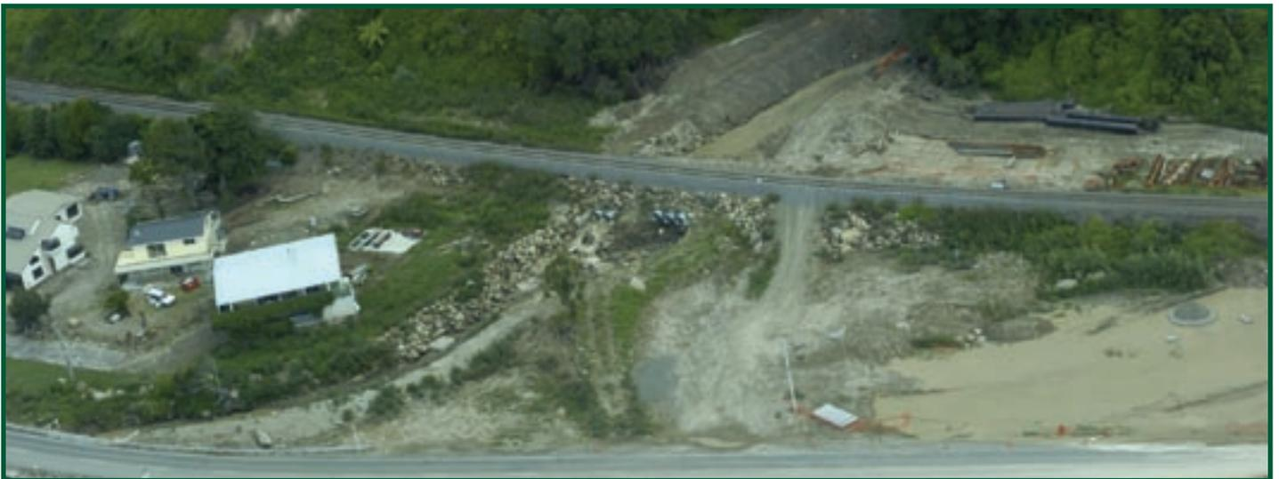
**FLOODPROOFING** – The new rail bridge will replace the temporary culverts in the centre of the photograph.
