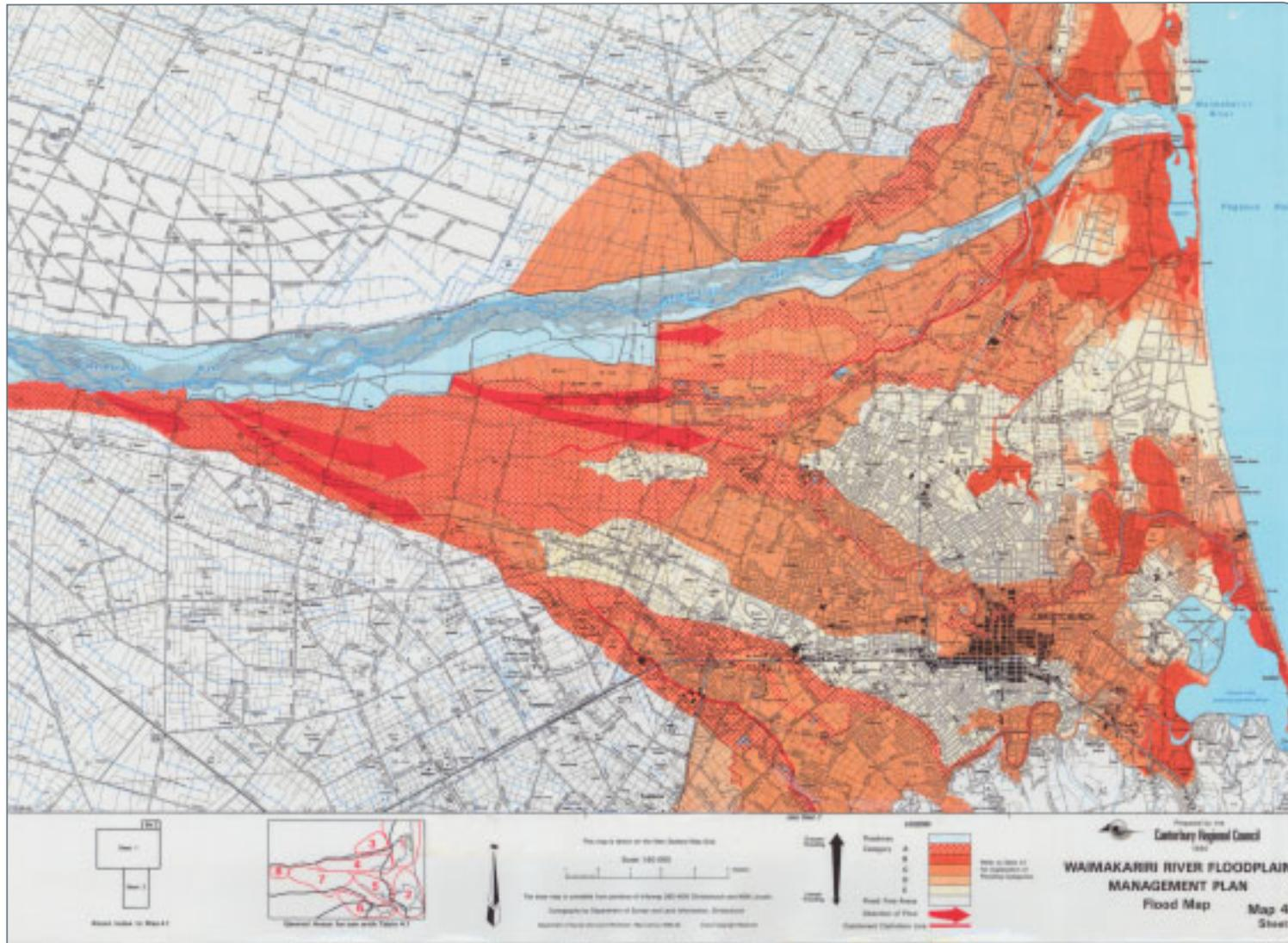
Flood hazard to Christchurch from the Waimakariri River, 1990. Flood protection works costing about \$30 million are proposed. The existing flood protection works and proposed improvements are expected to contain flood flows of 6500 m<sup>3</sup>/s – a one in 10 000 year event. Environment Canterbury estimates a major flood could inundate residential and industrial areas, causing up to \$2 billion worth of damage and affecting up to 300 000 people. *Environment Canterbury.*
