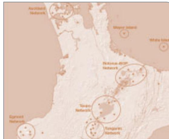
GeoNet's volcano-seismic network monitors volcanic earthquakes that indicate magma movement within the earth's crust. Volcanic earthquakes are distinguished from normal tectonic earthquakes by their slower vibration frequency. GNS Science.
