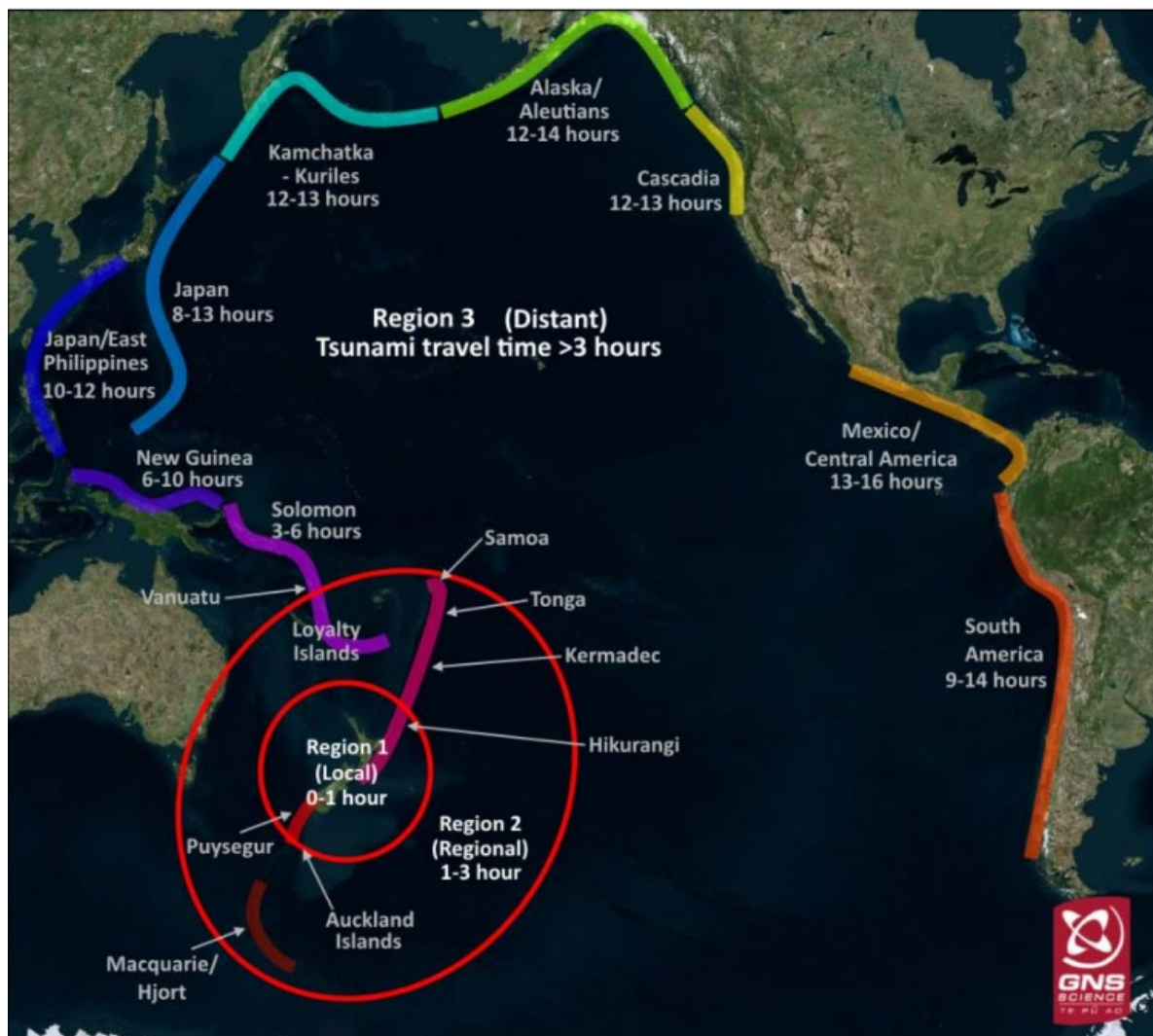
Figure 2 Tsunami source regions. Regions are based on the minimum travel time from source to the point of first arrival at the Aotearoa New Zealand coastline (including the Chatham Islands).
