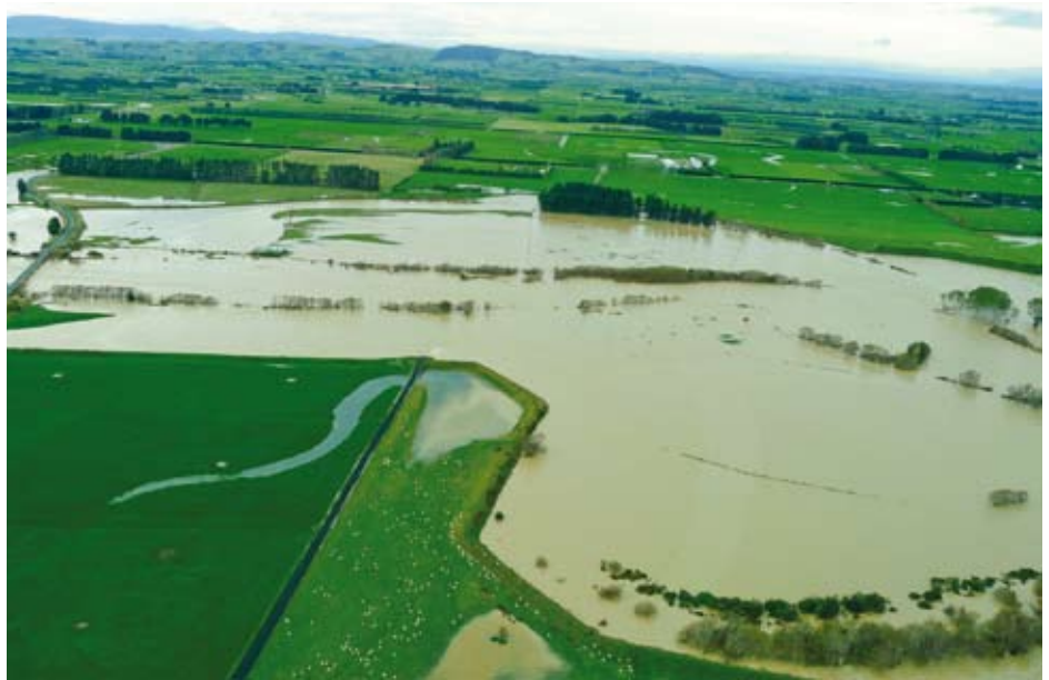
A comprehensive flood protection scheme kept the Oreti River contained within its stopbanks. While the river burst out of its channel (visible between the lines of willows in the centre of the image) the stopbanks protected thousands of hectares of farmland and several communities from inundation.
