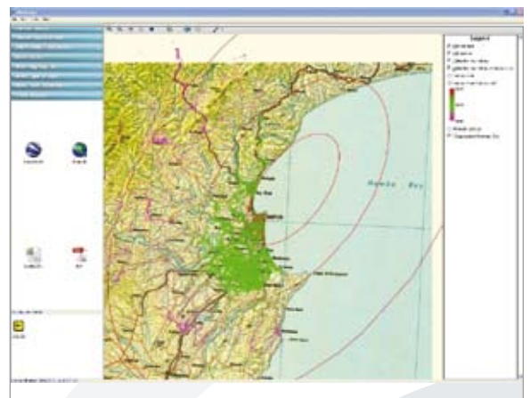
A screen-grab from the RiskScape application illustrating likely building impacts from an earthquake in Hawke's Bay
