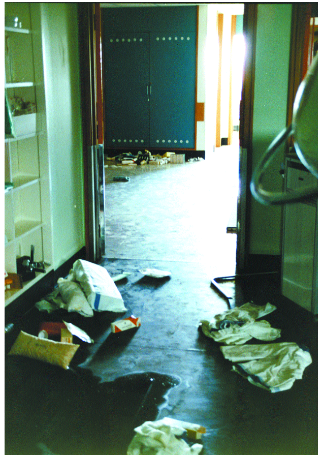
Unrestrained surgical supplies thrown to the ground at Whakatane Hospital during the March 1987 Edgecumbe Earthquake.
