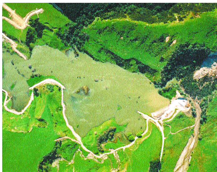
Figure 4.8. Te Ore Ore-Bideford Road, Masterton district. In August 1991, a large landslide, shown above, blocked the stream and the road and bridge were submerged for several months. A temporary route was constructed around the perimeter of the lake.
