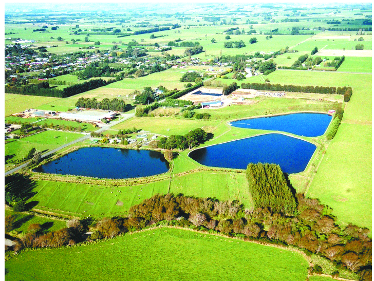
Figure 3.11. Carterton sewage treatment plant at Dalefield. The plant buildings in the centre of the photo are surrounded by the three treatment ponds. The Mangaterere Stream is in the foreground.
