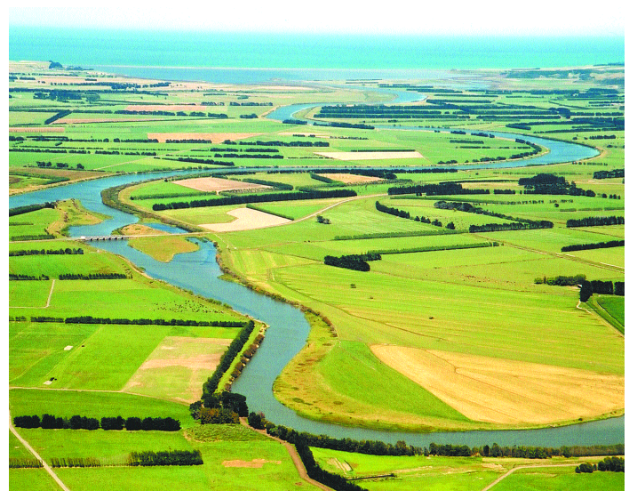
Figure 3.17. Lower reaches of the Ruamahanga River outlet from Lake Wairarapa. The Blundell Barrage combined flood protection structure and road bridge is located before the junction with the Ruamahanga River. All the flat land in the picture depends on stopbank protection and land drainage pumps.
