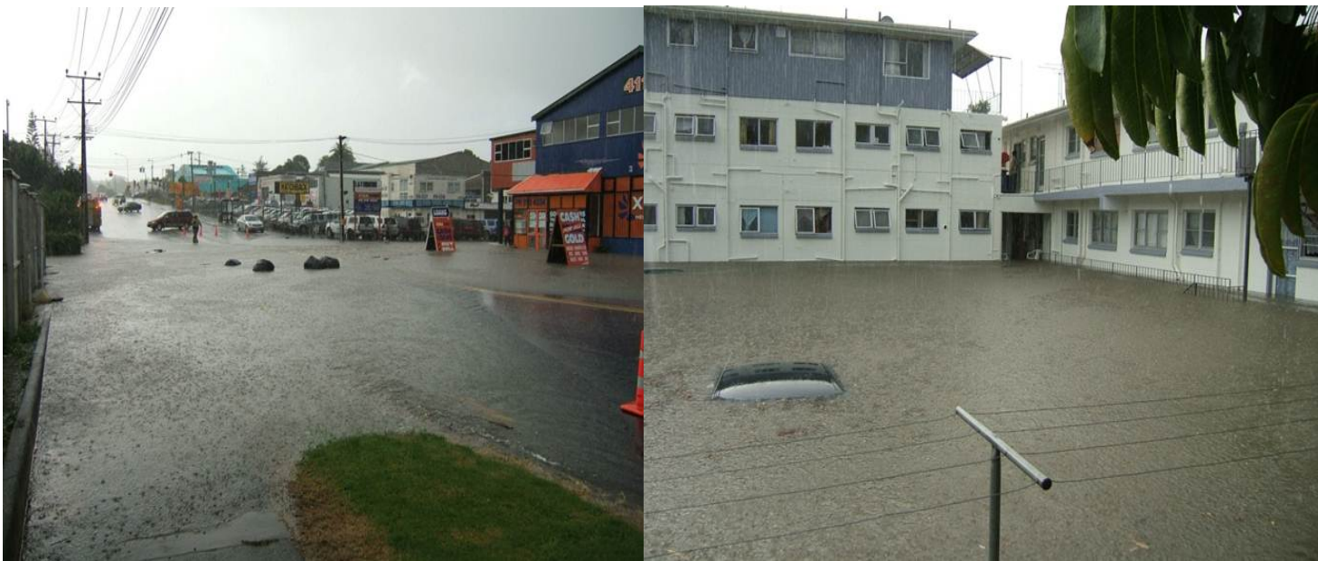
Figure 14. Flooding on Great North Road in 2012 (left image) following the collapse of a stormwater drain. The stormwater system was not adequate for more intense rainfall events, and the residual risk was realised when the system failed. (Right Image) Flooding in Cartwright Road, 2012. (note the height of floodwaters from the vehicle roof in the foreground). When natural drainage systems are replaced with piped infrastructure, the residual risk arises from events which supply more rainfall runoff than the pipes can carry. Source: Stuff news.
