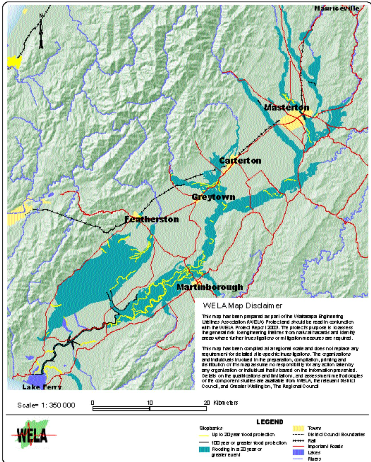
**Figure 2.38.** This figure shows the extent of flooding anticipated in a one in 20 and one in 50 year event. It provides for existing flood protection structures to function to their design standards during such events. Not all catchments would be expected to flood in any particular storm event.
