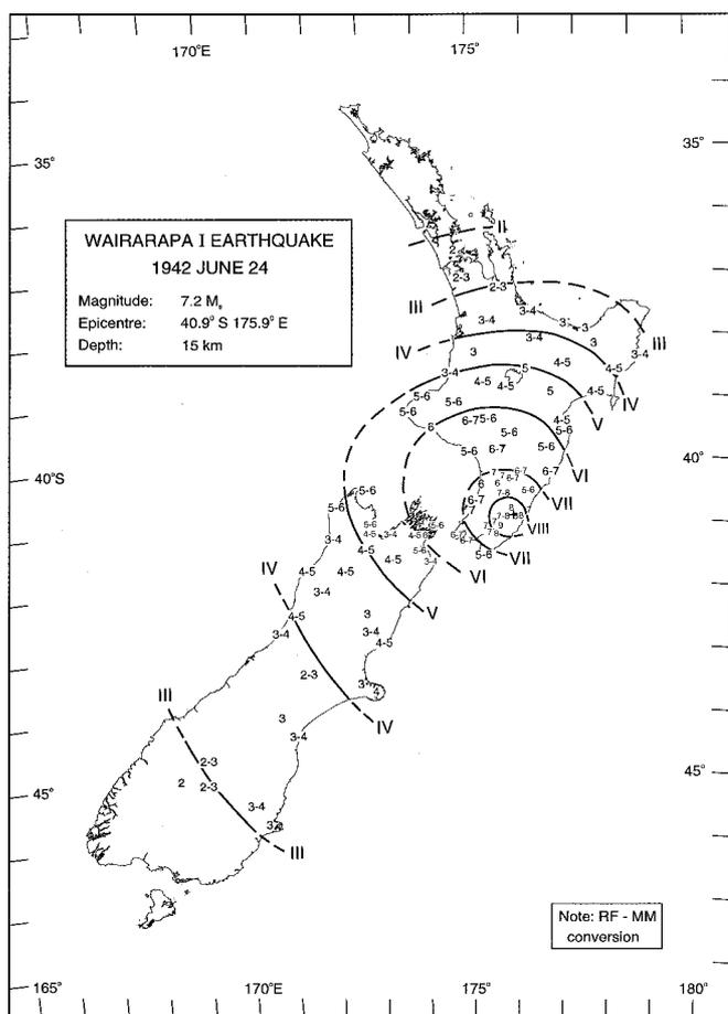
**Figure 2.5.** Isoseismals (lines joining points of equal shaking intensity) from the June 24, 1942 Masterton Earthquake. Source: Downes (2001).
