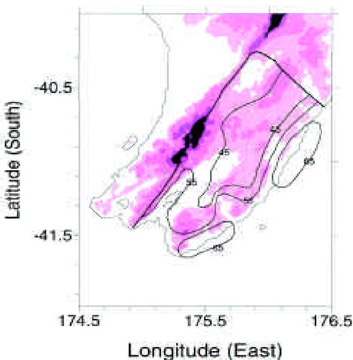
**Figure 2.28.** Contours of maximum wind gust speeds (metres per second) expected to be equalled or exceeded at average intervals of 142 years in the Wairarapa. Source: NIWA 1999-2000.
