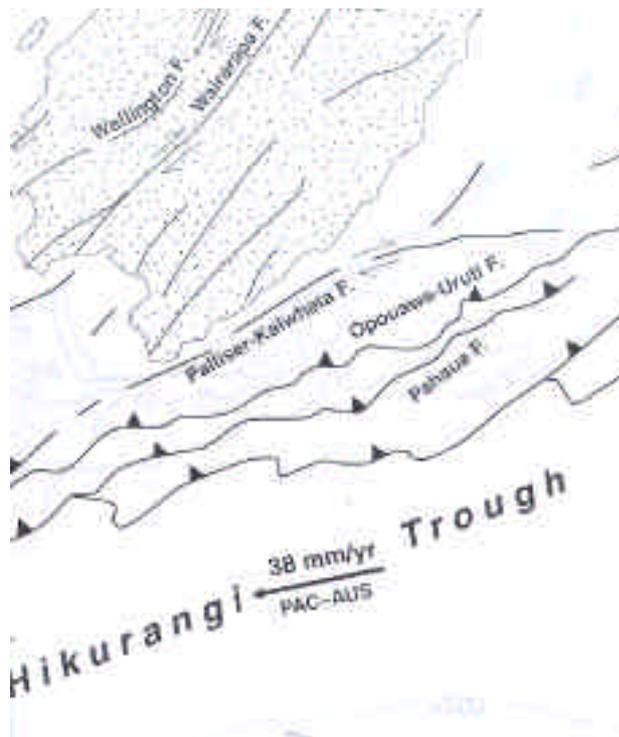
**Figure 2.21.** Map showing the Wairarapa's offshore faults and bathymetry (marine topography). Tsunamis could be generated from movement of the faults or landslides in the Cook Strait Canyon or Hikurangi Trough. Source: Barnes and Audru (1999).
