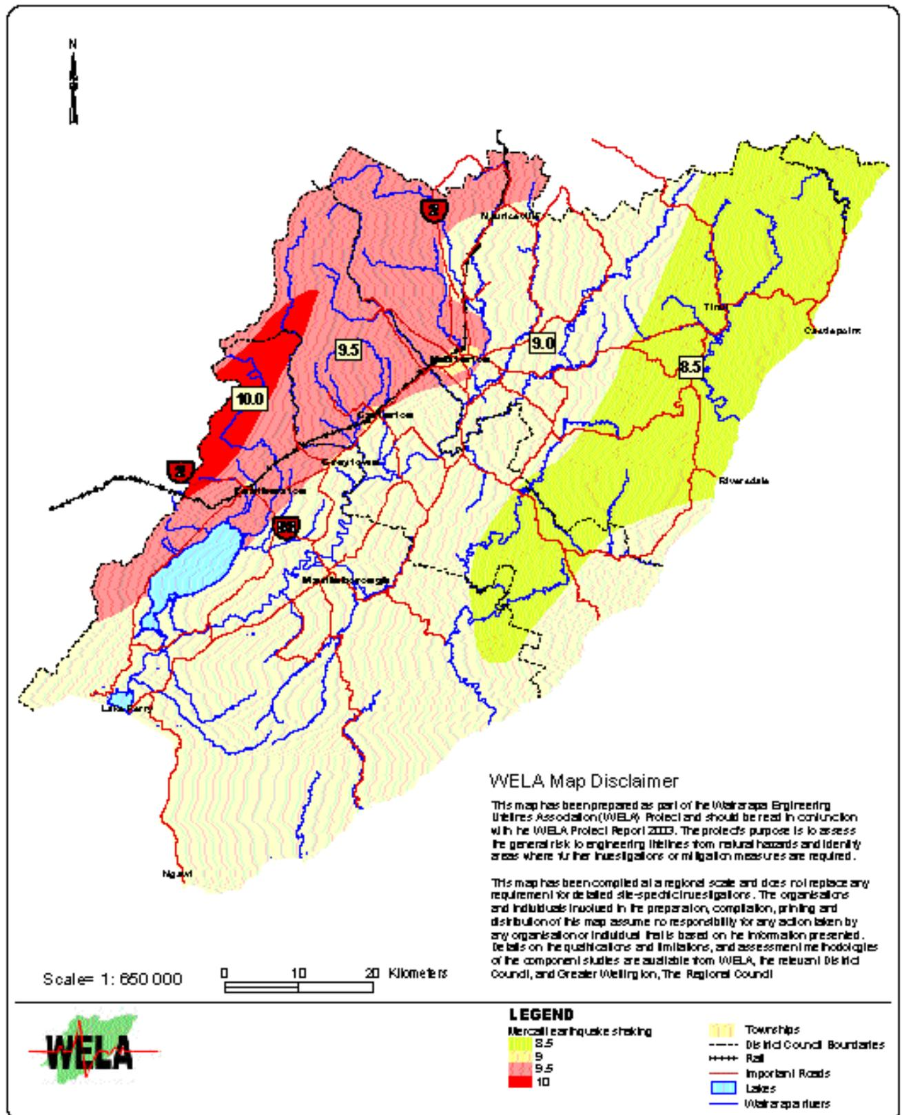
**Figure 2.3.** Predicted Modified Mercalli Shaking in the Wairarapa for a one in 475 year earthquake event. The predicted values of MMI are for average ground conditions, such as the firm alluvium that underlies many of the towns in the Wairarapa.
