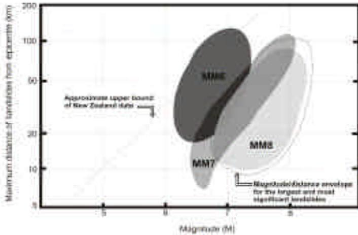
**Figure 2.43.** This figure highlights the shaking intensity that has triggered landslides in New Zealand. The shaded envelopes show the MM intensities (MM VI to MM IX or greater) at which landslides have occurred in relation to earthquake magnitude and distance from source. *Source:* Hancox et al, 1995.
