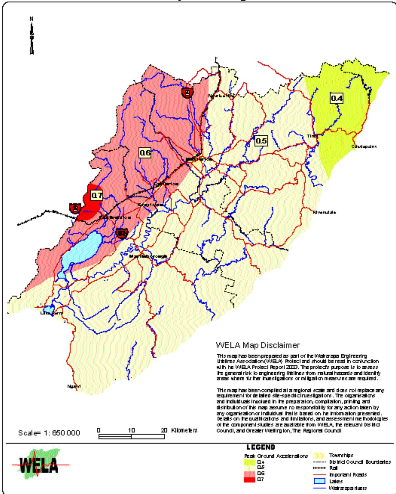
**Figure 2.4.** Predicted peak ground acceleration in the Wairarapa for a one in 475 year event. The predicted values of PGA are for average ground conditions, such as the firm alluvium that underlies many of the towns in the Wairarapa.
