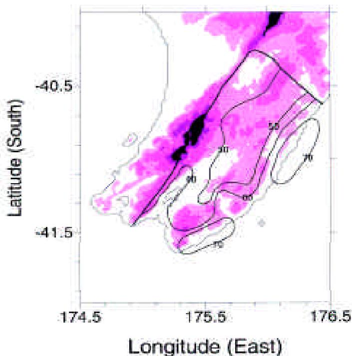
**Figure 2.29.** Contours of maximum wind gust speeds (metres per second) expected to be equalled or exceeded at average intervals of 475 years in the Wairarapa. Source: NIWA 1999-2000.
