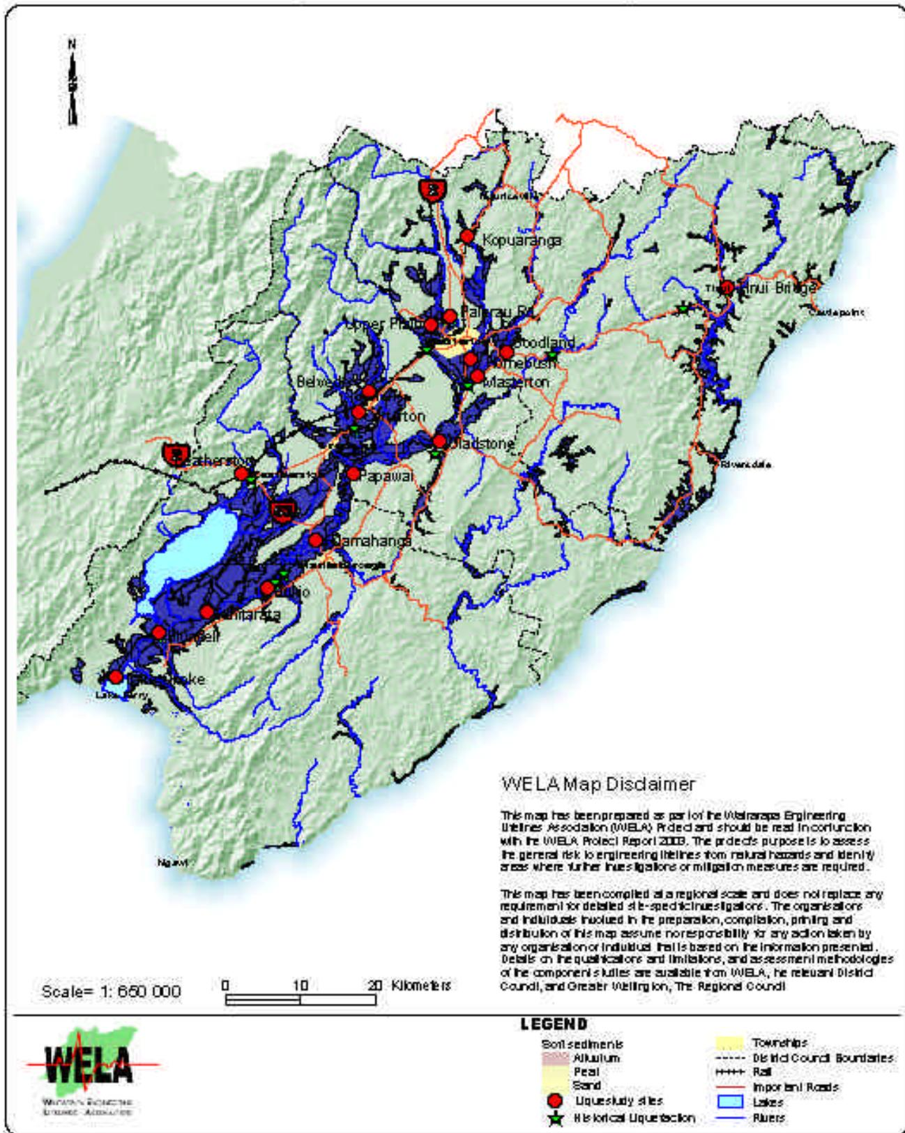
**Figure 2.10.** Map indicating potential liquefaction in the Wairarapa. The soft sediments shown on the map represent areas potentially at risk. The map also shows sites of historical liquefaction, and the sites studied by Wick in 2000. Note: not all the soft sediments on the map are susceptible to liquefaction. Some of the sites of historic liquefaction are not in areas of predominantly soft sediments.
