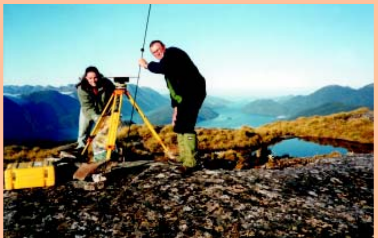
Surveyors Ashley MacFarlane and Kim Saunderson measure the height of the GPS antenna above a survey mark, at the start of GPS measurements in Fiordland.
