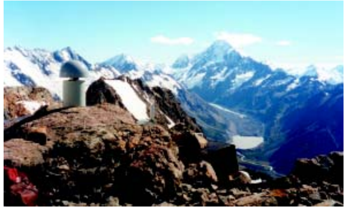
This continuous GPS site in the Southern Alps network is on Annette Plateau above the Tasman Valley, near Mt Sefton and Mt Cook. Measurements at this site are helping us to understand the growth of the mountains.
