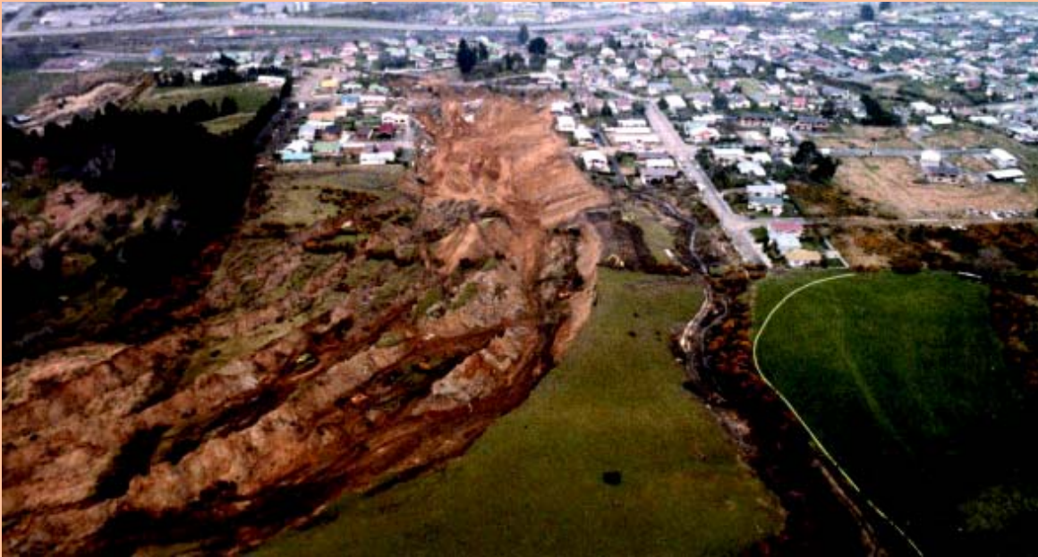
Aerial view, looking south, of the Abbotsford Landslide on 12 Aug 1979. In the foreground sharp ridges and deep cracks up to 15m deep can be seen within the extensive head scarp graben. In the distance earth moving equipment have smoothed off the head scarp and partly infilled the graben to stabilise the area. (Photo: Graham Hancox, GNS)
