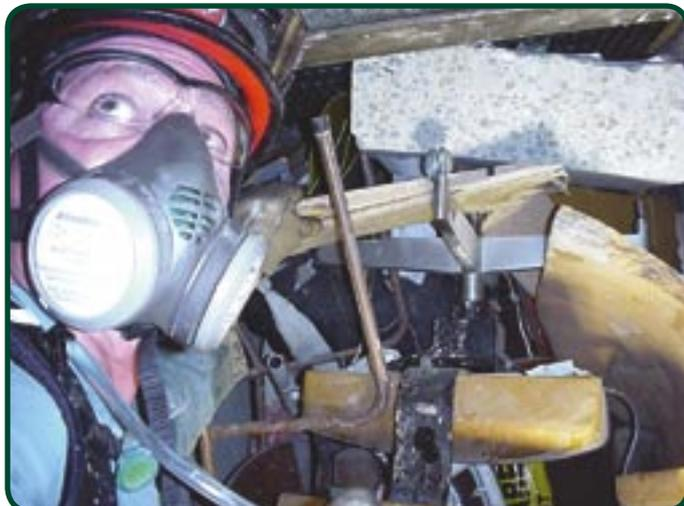
Tunnelling through a pancake collapse simulator to exercise the rescue process in an apartment building collapse scenario.
