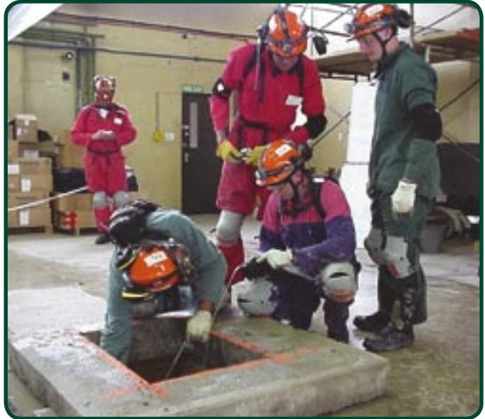
Taskforce technicians using atmospheric monitoring equipment to check air quality before entering a confined space.
