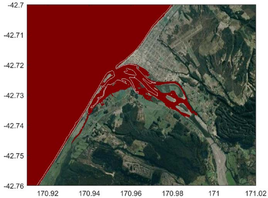
Figure 4.37 The inundation area produced by tracing the grids that are connected to the sea and lower than 2 m above the MHWS level of 1.1 m for Hokitika.
