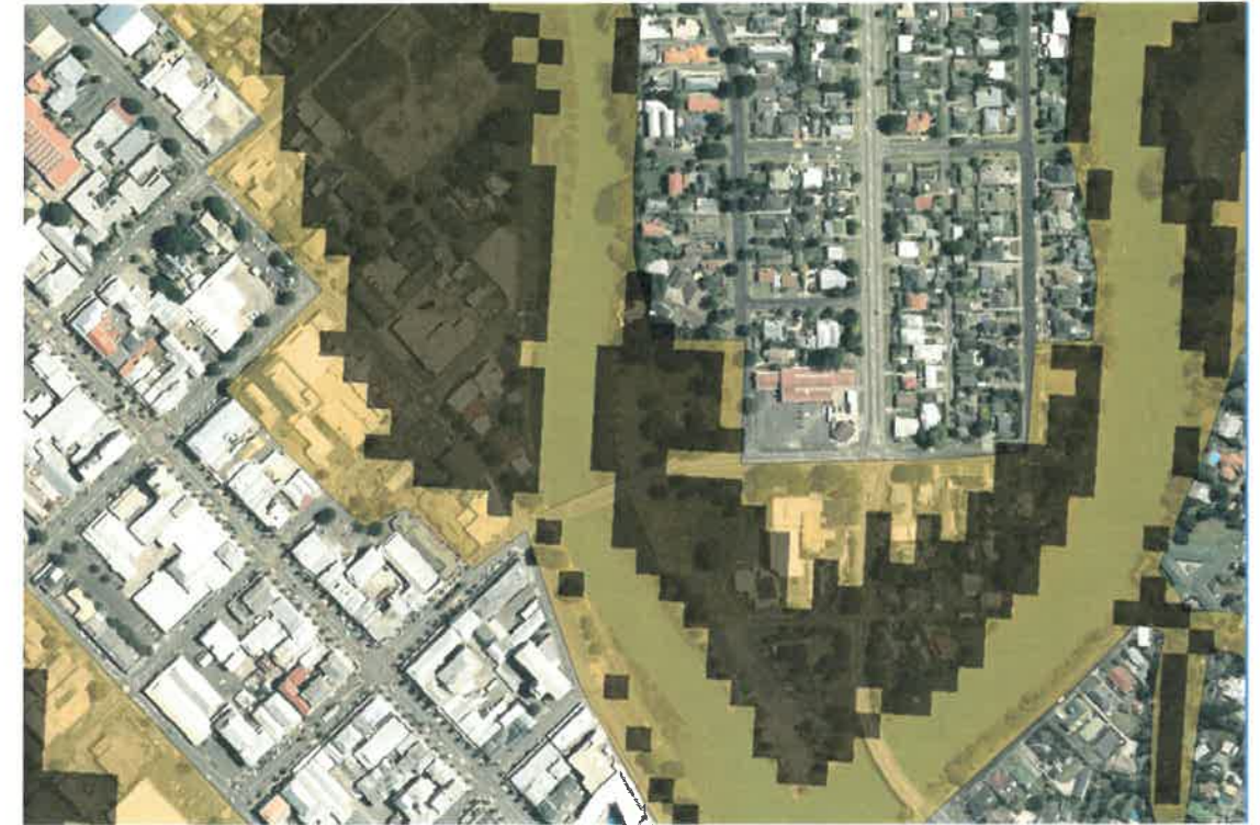
Figure 6.1 Example of zone adjustment. The darker shading represents the simulated inundation extent for the orange zone scenarios. The Orange shading shows the adjusted Orange zone.
