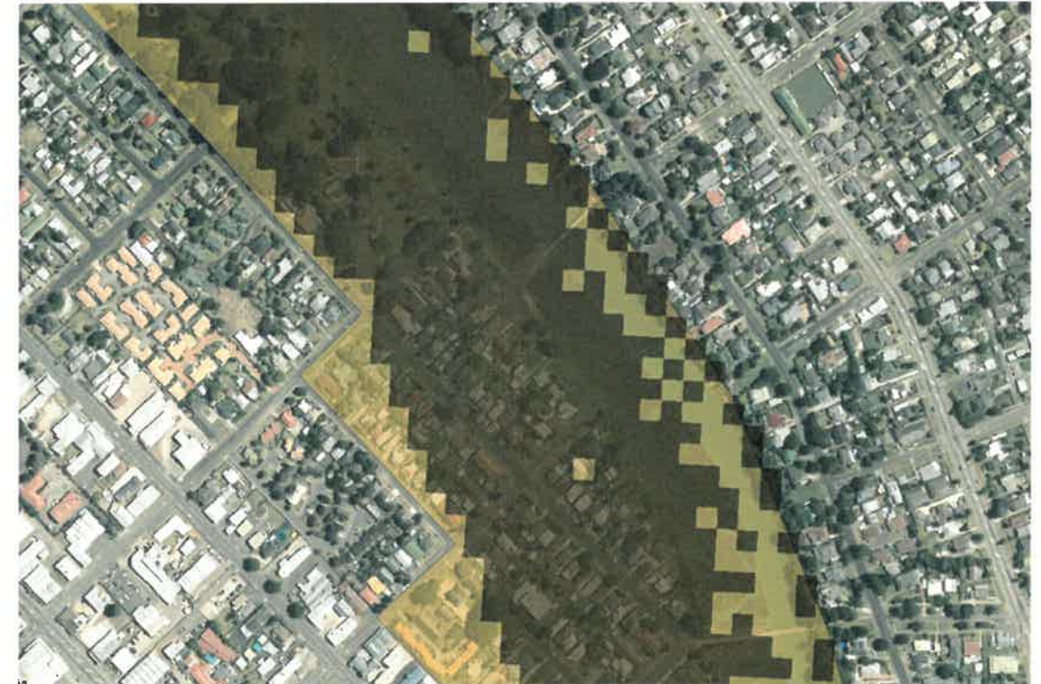
Figure 6.2 Example of zone adjustment. The black shading represents the simulated inundation extent for the orange zone scenarios. The Orange shading shows the adjusted Orange zone.
