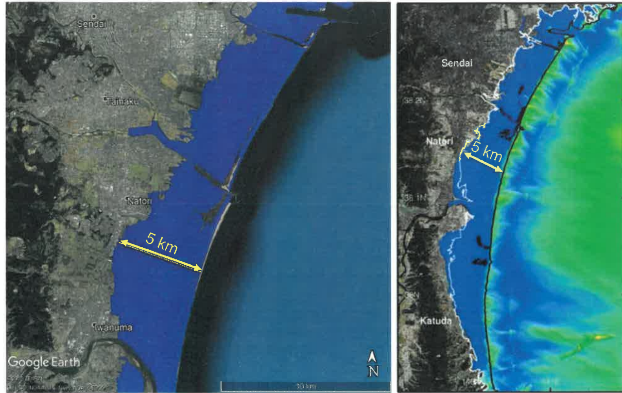
Figure 3.9 (left) close of up the inundation extents over the Sendai Plain. The yellow line across the inundation zone measures 5.2 km. (right) The MOST/ComMIT model results of Wei et al., (2013) compared to the measured inundation extents (white line).
