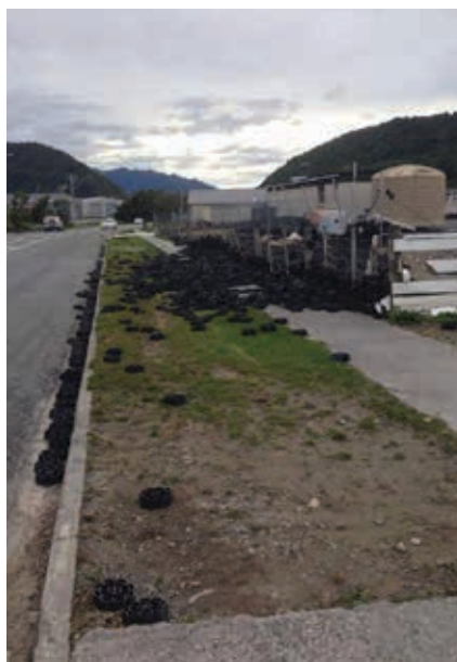
(Left) Plastic discs from treatment plant. The plastic discs are used to grow bacteria in the treatment plant. Fortunately the plant had not been commissioned, and the discs were clean.
